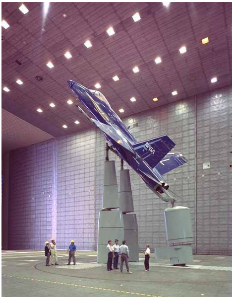
F/A-18 High Alpha fighter testing high angle-of-attack aerodynamics in 80x120ft W.T.
