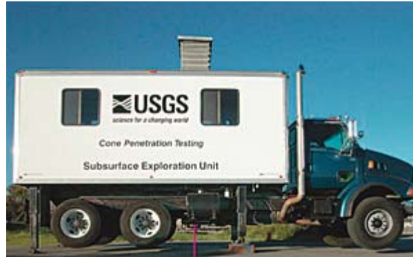
U.S. Geological Survey truck uses cone penetrometer to record soil liquefaction characteristics.
